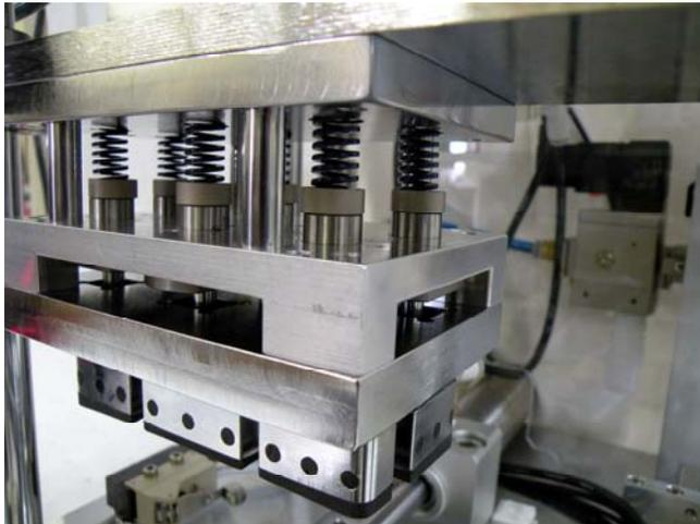
**Basic press machine with a spring loaded head for assembling and pressing knobs onto a body. All of the spring loaded heads like this use Misumi's springs, bearings, posts, and washer caps.**
